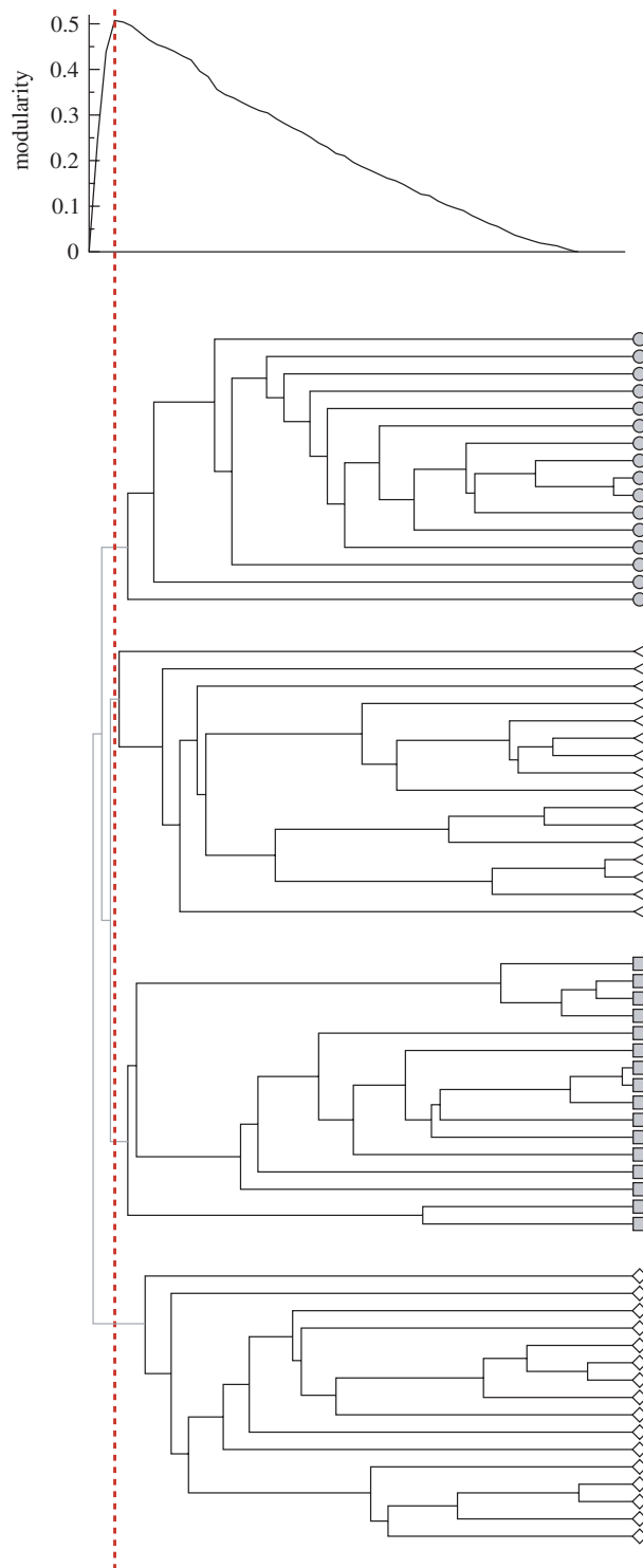
Fig. 7.3. Modularity Q (top panel) and dendrogram (bottom panel) obtained by the application of the GN algorithm to a computer generated modular random graph with 64 vertices and 256 edges. The random graph has been generated, as described in the text, by dividing the nodes into 4 groups of 16 nodes each (respectively empty circles, full circles, triangles and squares) and by considering z_{in} = 6 , z_{out} = 2 . The peak in the modularity (dotted line) corresponds to a perfect identification of the 4 communities.
